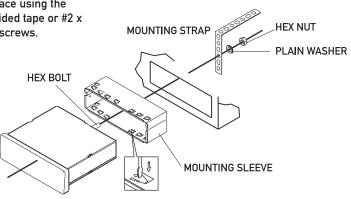
TYPICAL FRONT-LOAD DIN MOUNTING METHOD
